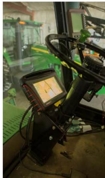
GPS and precision technology in farm equipment allow farmers to use pinpoint accuracy when applying fertilizer and pesticides. Photo courtesy of United Soybean Board
