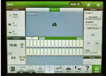
The IntelliDrive system is directed by proprietary JCA Electronics software that displays as an interactive on John Deere split screens or any monitor.
