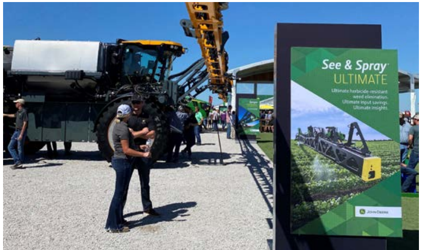
John Deere See and Spray™ technology works by having cameras on the machine scan the field, while a computer processor identifies the crop, like soy, and sends a signal to the nozzle to spray all unwanted plants, such as weeds.
