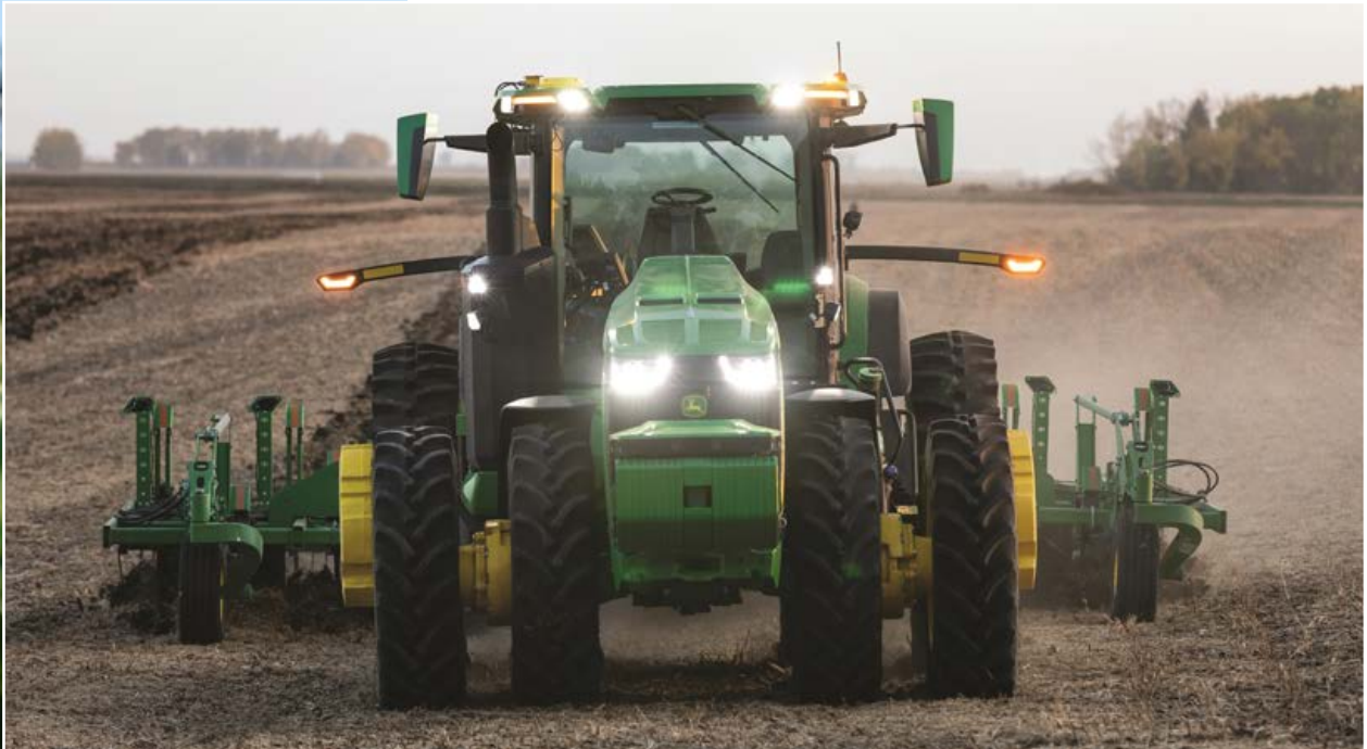
Technology is taking over the farm, and other autonomous systems aren't far behind. Pictured here is a driverless John Deere tractor, which is expected to hit the market this fall. Photo credit: John Deere
