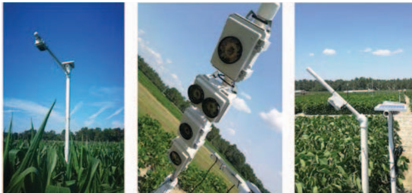
Cameras mounted in the field. Left: Pole camera in corn plot. Middle: Set of cameras tested in the field. Right: Pole camera in soybean field
